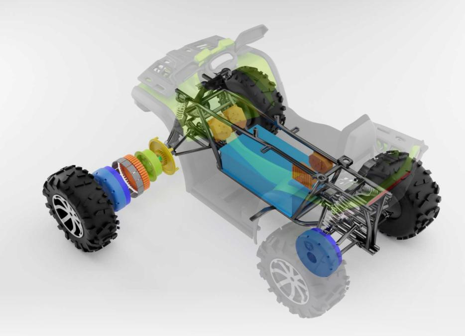
**Power** - The direct-drive hub motors enable the vehicle to achieve up to 50 horsepower at peak power and 800 Nm of torque at the wheels.
